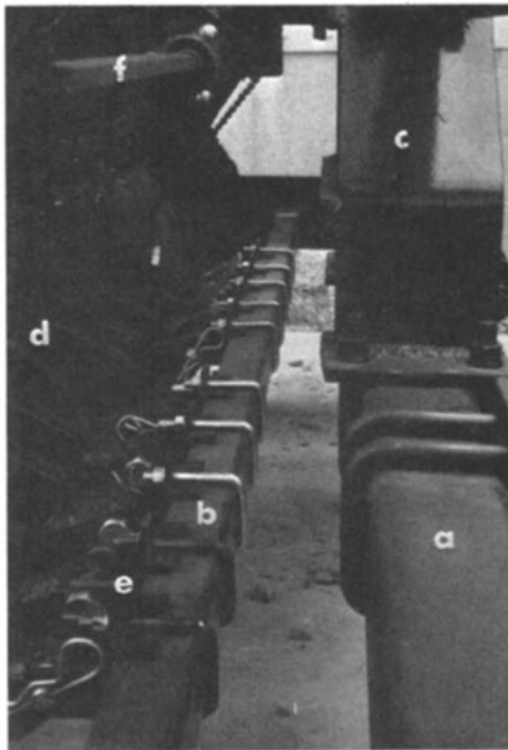
Fig. 6. Front tool bars: a. 102-mm square tube, b. 51-mm square tube, c. third link yoke, d. grain drill double disk openers, e. clamps, f. hex shaft.
