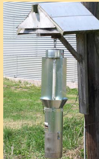
This trap location is also not ideal because there is a building within 200 ft of the trap on one side, but it is acceptable if there are no other obstructions in a 180° radius of the trap within 200 ft.
