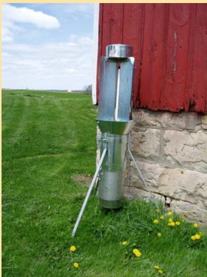
This blacklight trap location is not ideal because one side is blocked by a building, however it is acceptable because it is open at least 180° around the trap.
