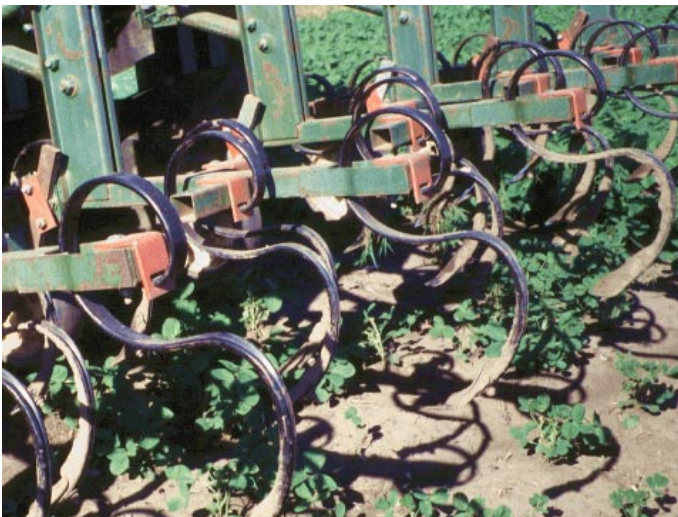
The S-tine (pictured above) gives more vibrating action than the C-shank.
