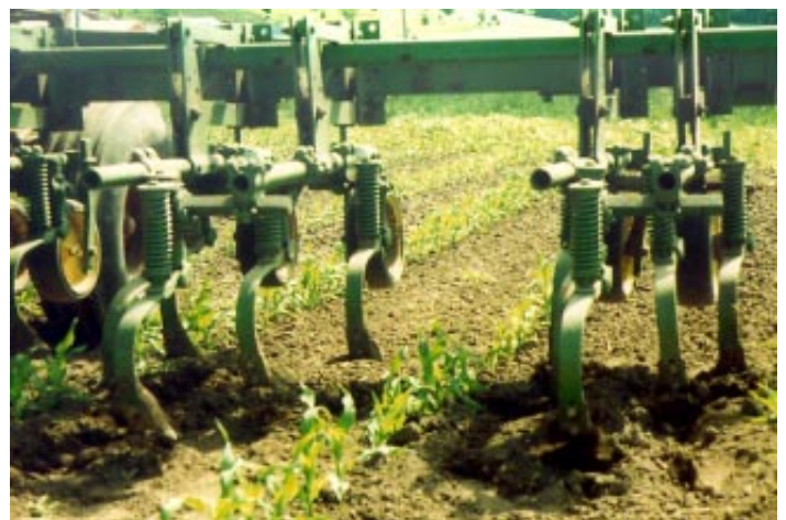
C-shanks in gang assemblies connected to the tool bar.
