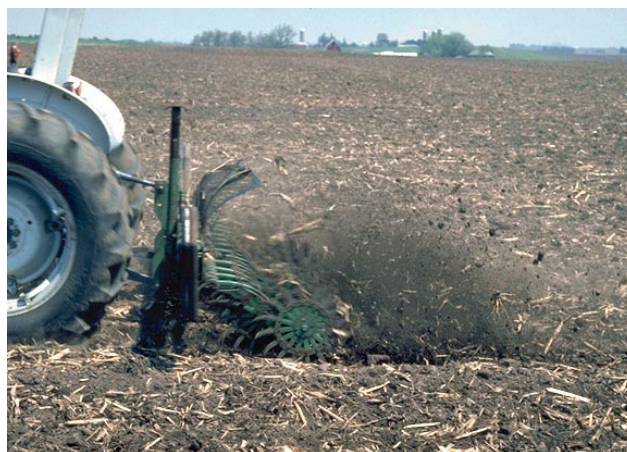
A rotary hoe stirs the soil and flicks out tiny germinating weeds and seeds.
